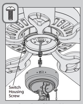
Partially install two of the switch housing screws found in the ≡ hardware bag.
